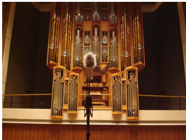
Figure 4 – Exp2 with windscreen hovering over a Soundfield MkV at the Holiday Organ Concert at Bates Recital Hall. One observer noted the Experimental Microphone “looks like a varmint on a stick.”
